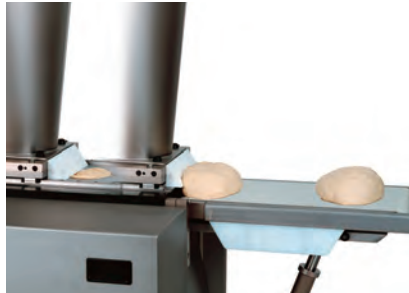
Vacuum scaling system with built-in vacuum pump.
